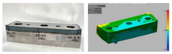
Figure 3. Laser heat treated trim inserts (approximate dimensions of 7" x 4" x 3", base material 4140) demonstrate distortion of less than 10 microns and hardness of 55–57 HRC.
