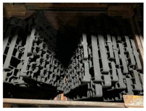
Figure 7. Typical scrap alloy trays and grids (Source: Castalloy Group)
