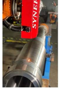
*Figure 5. Laser heat treating the OD of large industrial shaft used in paper mills*
