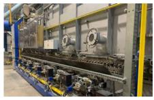
Indirectly heated roller hearth furnace
