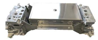
Figure 7. (left) Robot loading of combined thru-process system with engine block into BSN rotary T6 furnace. The thermal barrier is designed with a combination of thermal insulation technology capable of fitting in the engine block cavity. (right) Thermal barrier mounted within engine block assembly. (Source: BSN Thermprozesstechnik GmbH)
