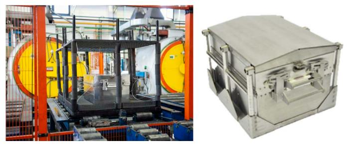
Figures 5. (left) Thermal barrier being loaded into LPC batch furnace with TUS frame as part of temperature uniformity survey. (right) Thermal barrier shown with independent quench deflector providing protection during the high pressure gas quench. (Source: PhoenixTM)
