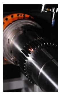
*Figure 4. Laser heat treating of gear tooth profile*
