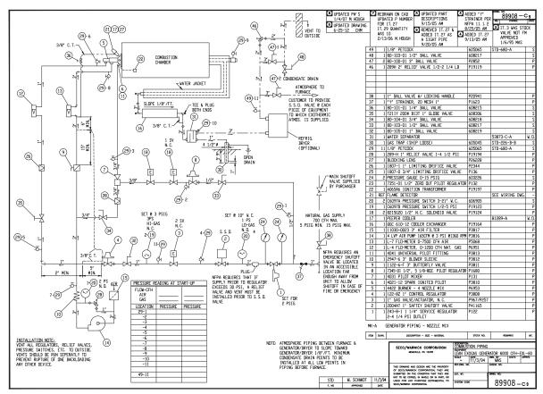
Figure 3. Lean Exo generator schematic flow diagram (Source: SECO/WARWICK)
