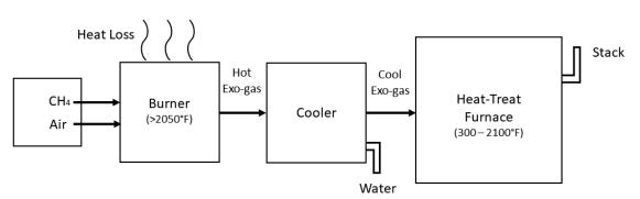
Figure 1. Schematic flow diagram showing Exo production, cool down, and its use. (Source: Morris, "Exothermic Reactions," 2023)
