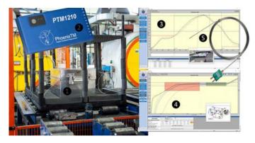
Figure 2. PhoenixTM thru-process monitoring system. (1) The thermal barrier protects internal multi-channel data logger, (2) the field test instrument, (3) the product thermal profile view, (4) the temperature uniformity survey (TUS), and (5) short nonexpendable mineral insulated thermocouples. (Source: PhoenixTM)
