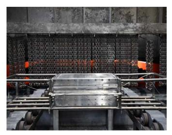
Figures 3. Temperature uniformity survey of a continuous furnace using the plane method applying the PhoenixTM thru-process monitoring system. The data logger travels protected in a thermal barrier mounted on the TUS frame performing a safe TUS at four points across the width, which is impossible with trailing thermocouples. (Source: Raba Axle, Györ, Hungary)
